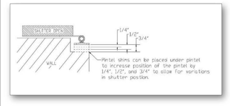
All hardware is made from 304 Stainless Steel and is Powder coated Black finish.
