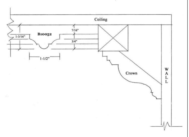
This sketch illustrates a solution for terminating our B10052 and C10052 ceiling panels up against the walls of a room using the block & crown method. Of course, this works only in rooms that don't have crown moldings already in them.
