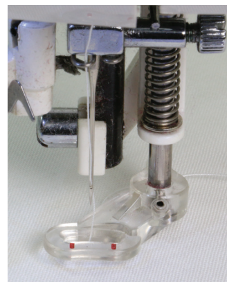
Clear plastic darning foot comes with many machine brands. It bounces a lot, and it's hard to see the needle.
