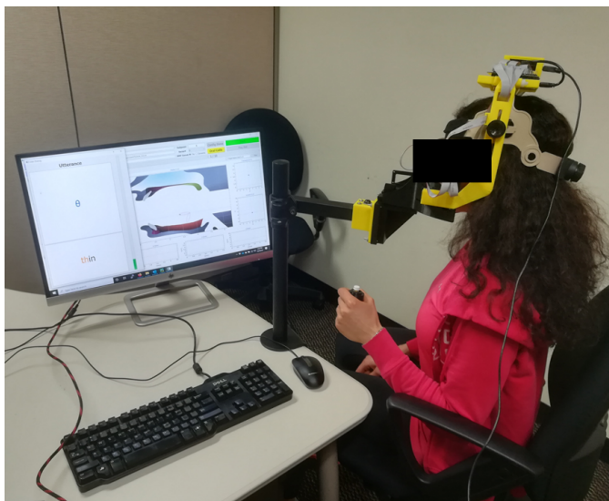
Fig. 3. Illustration of a subject using our tongue tracking system during a data collection session.
