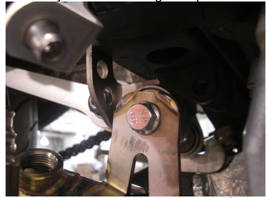
Bolt mounting tab to bracket on underside of chassis using supplied M8 flange nut and M8 x 35mm hex flange bolt.
