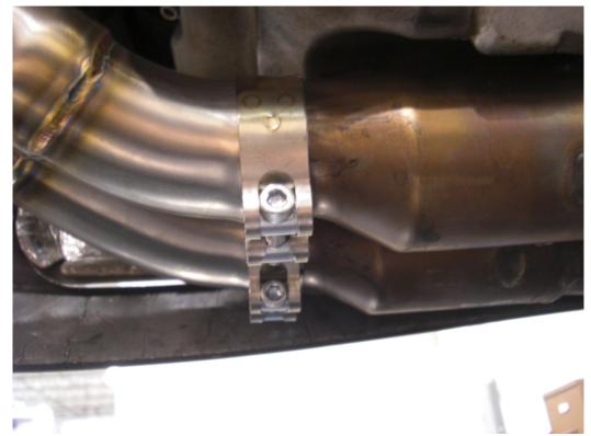
You can now slip your muffler box eliminator (with barrel clamps installed) onto the stock header unit. \*Note: We recommend that you use some high temp. sealant on this joint.
