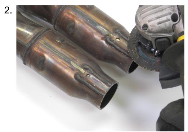
Grind area smooth approximately one inch up from where cut was made. This will provide you with some tangent to clamp the muffler box eliminator to.
