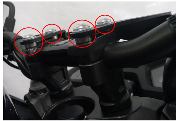
Position of the steel spacers
