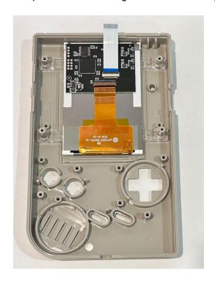
**STEP 7:** Place buttons first and pads second in the shell. Make sure everything goes in smoothly so buttons work properly.
