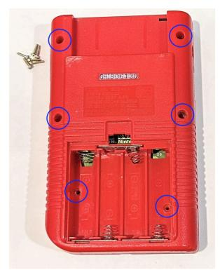
STEP 1: Remove back of DMG shell with a Y2
