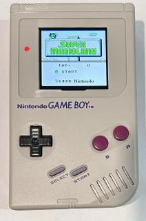
**STEP 14:** Install self-adhesive lens on top of the LCD. Make sure everything is dust free because removing the lens once installed can be difficult.
