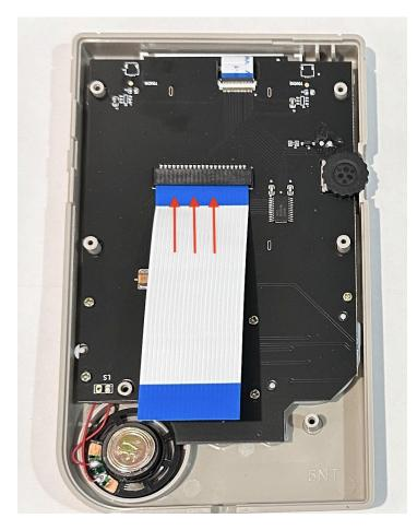
**STEP 10:** Place connecting cable into the back port of the front board. Then push up as much as possible. This will make sure the cable does not loosen. Most issues that occur are because the connecting cable is not properly installed.
