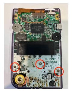
**STEP 12:** Screw in the 2-3 Phillips screws back in and place the top power switch. Make sure the screws are not too tight. It can cause small white dots on the LCD or damage the board if screwed in too tight. Then place the back shell on the system.
