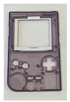
**STEP 5**: Prepare your shell on a soft surface to avoid scratches and attach an adhesive pad around the inner LCD frame.
