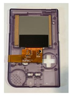
**STEP 6:** Remove the white protective paper on the adhesive and place the NEW LCD on top The screen will be smaller than the old LCD so you might see a little space on the side.
