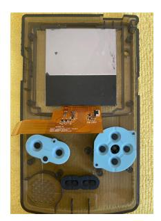
**STEP 6:** Remove the white protective paper on the adhesive and place the NEW LCD on top The screen will be smaller than the old LCD so you might see a little border outside the bezel. Place the insulation film on both the LCD and PCB board.
