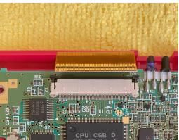
**STEP 4:** Lift up the ribbon and remove it from the adapter. You can remove the motherboard from the system. This is the only part you will need from the original GBC.
