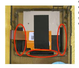
centered. It should come with enough material in case you make a mistake. You should put stoppers in these 3 areas. Taping down the ribbon is not necessary.
