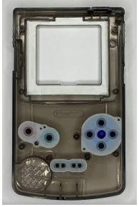
**STEP 5**: Prepare your shell on a soft surface to avoid scratches and place buttons and pads and attach adhesive pad around inner LCD frame. (If you have an older version of the kit you will not have the adhesive pad, you can skip that potion of the installation.)
