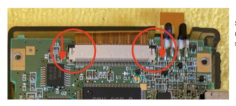
**STEP 10:** Plug top ribbon into the GBC motherboard. And push the side tabs down to secure the ribbon into the port.
