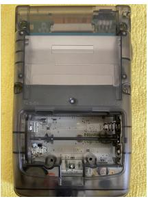
**STEP 12:** Screw in the 2-3 Phillips screws back in and place the side power switch. Make sure the screws are not too tight. It can cause small white dots on the LCD or damage the board if screwed in too tight. Then place the back shell on the system.
