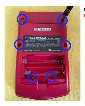
**STEP 1:** Remove the 6 tri-wing screws with a Y2 tri-wing screwdriver. **DO NOT THROW AWAY SCREWS.**
