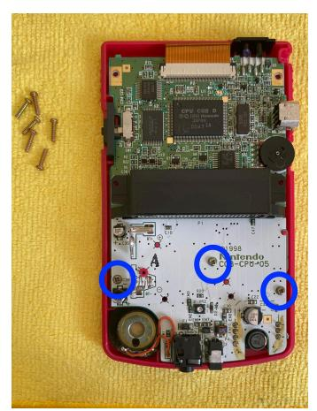
**STEP 2:** Remove backplate and you will see 2-3 screws holding down the motherboard. With a 00 Phillips screwdriver remove them and put them to the side.
