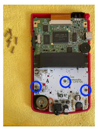
**STEP 2:** Remove backplate and you will see 2-3 screws holding down the motherboard. With a 00 Phillips screwdriver remove them and put them to the side.
