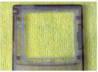
**STEP 6**: Attach the adhesive pad to the edges of the LCD frame of the shell and remove the white protective paper, if necessary you can cut it to size to fit the trimmed area.
