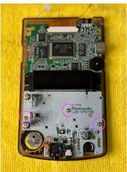
**STEP 13:** Remove the adhesive cover off the touch sensors and place them at the top of the shell in the picture shown. If you need to use the IR sensor, place it in a different location. Also place the power switch button into the power switch.
