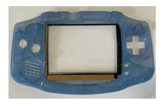
**STEP 7:** Place the LCD on the shell and place the insulating film over the back of the LCD (Make sure to place because it can cause issues.)
