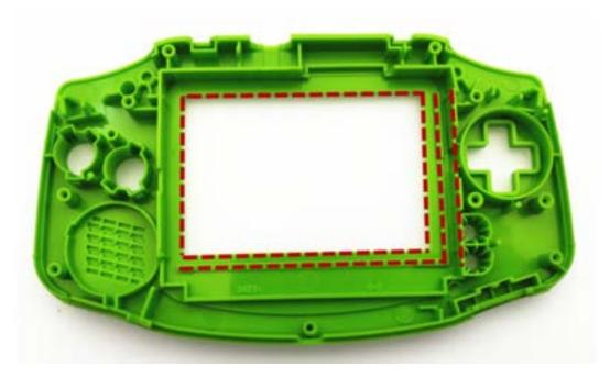
**STEP 5:** Place the adhesive sticker along the frame of the front of the shell.
