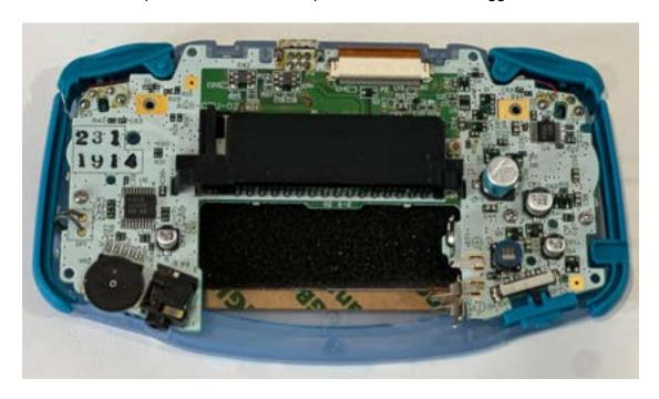
**STEP 14:** Attach the back plate of the shell and we recommend you test the system now before you close it up. Screw in the big screws in at the spaces shown below. Make sure for the screw in the battery compartment (green circle) you use the smaller screw as a big screw may damage the shell.
