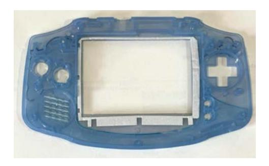
**STEP 6:** Remove the adhesive cover and place the 2 plastic separators on the area indicated below. Some Pre-trimmed shells come molded with brackets already on them. If that is the case then this step is not necessary. This is only necessary if your shell is hand-trimmed.
