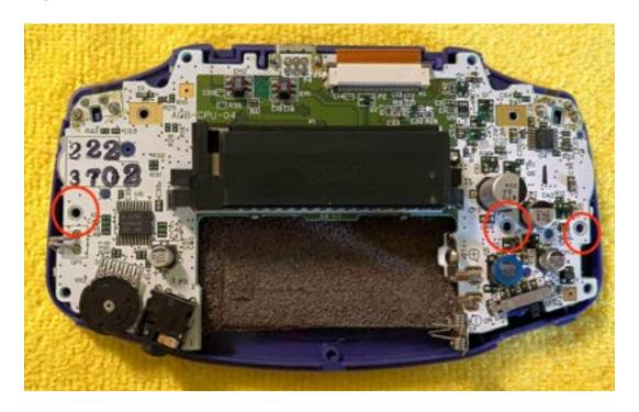
**STEP 3:** To separate the motherboard from the LCD, lift the 2 side notches and then lift the ribbon out of the port.
