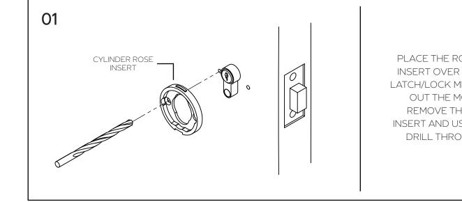
PLACE THE ROSE CYLINDER ROSE INSERT OVER THE PRE INSTALLED LATCH/LOCK MECHANISM AND MARK OUT THE MOUNTING POINTS. REMOVE THE CYLINDER ROSE INSERT AND USING A 6MM DRILL BIT, DRILL THROUGH THE MARKED
