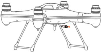
A line drawing of a drone from a top-down perspective. A small screw is located on the underside of the drone's central body, indicated by a red dot. | <p>1. Loosen the screw on the underside of the drone.</p>                                                                                                                                                                                                                                                                                    |
