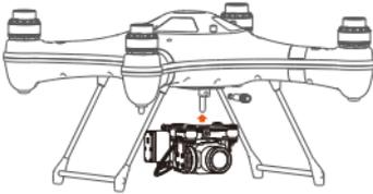
A line drawing of a drone with a gimbal assembly being attached to the bottom plate. A red dot indicates the alignment point for the gimbal.          | <p>2. 3. Mount the Gimbal onto the bottom plate, and secure it with the fixing screw.</p>                                                                                                                                                                                                                                                    |
