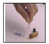
squeeze the plastic tube to crush the ampule. This will decrease the chance that the powder will be blown off the tip when the ampule is broken. Turn the ampule downward and gently squeeze the tube to force the pink liquid into the fiber tip.
