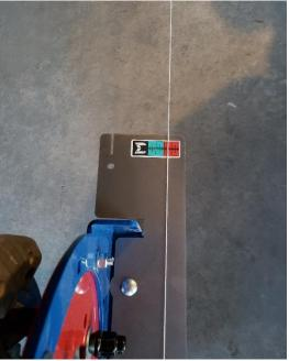
Remember that making adjustments to one thing will effect others. This system was designed to have minimal error if the steering is not perfectly straight but it is still a good idea to make sure the steering is pointed straight. This can be done by noting where the string crosses the calibration stickers on the front toe plates.
