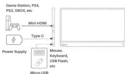
Please ensure Type-C charaina port is connected to power source under HDMI settings since power source is supplied via Type C connection only.
