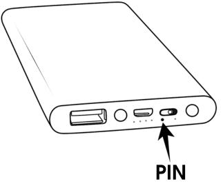
Insert a pin in the reset hole to reset the device. Keep it pressed for a few seconds.
