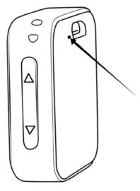
When the device stops working, please use a pin or needle to press the reset hole on the back of the device, then the device would be restored.
