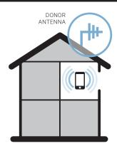
Install **Donor Antenna** where the mobile device receives this signal.
