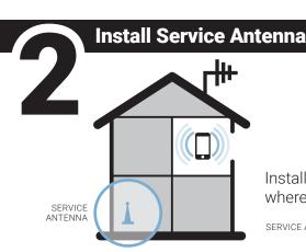
Install **Service Antenna** where coverage is needed.
