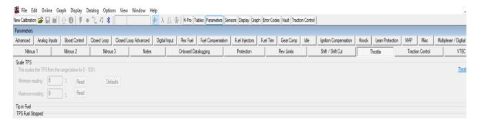
Lastly, select the "VTEC" tab and be sure that "VTEC oil pressure switch enabled" is NOT selected.
