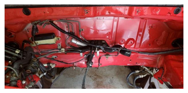
The above picture is with the engine removed. We are going to remove the driver-side cable. This kit re-uses the <u>passenger cable</u>. If you need to also replace the passenger side cable, we do offer them with a 25% increase in thickness to increase the strength.
