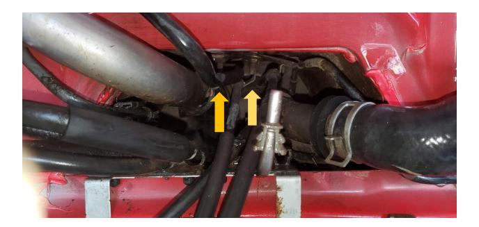
There are 2 nuts with studs in the middle of the car where the shift cables exit from the shifter. Undo the nuts to remove the brackets for the cables. The one on the driver side is for the driver side cable but is nearly inaccessible until the passenger side bracket is removed. These are 10mm nuts. Once removed you can take the bracket off. Now go to the interior of the car and remove the seats and center console.
