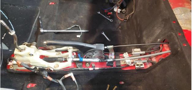
Re-attach the shifter, replace the retainer clip, and install the new bracket (see above picture).
