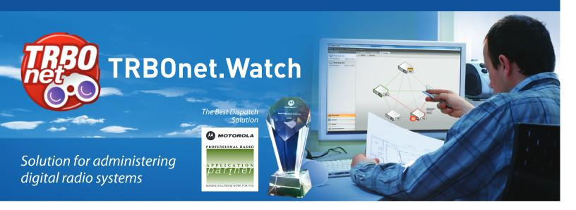
**TRBOnet.Watch** is a client-server Windows application that monitors all traffic on Motorola MOTOTRBO™ IP Site Connect, Capacity Plus systems or single repeaters. It displays transmitted GPS, ARS, Voice, Text Messages, System and User data with RSSI, source and destination radio ID's, Peer ID's.TRBOnet Watch helps to balance a channel loading, define and solve problems in a radionetwork.
