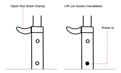
When you hear it click, close Stem Clamp to lock. Make sure the Handlebar is secure.
