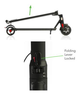
To fold the Slate, loosen the Folding Lever by sliding the Red Clip up and lowering the Folding Lever all the way down. Lower the Handlebar and Stem down towards the Deck and then connect the Hook to the Loop on the Rear Brake.
