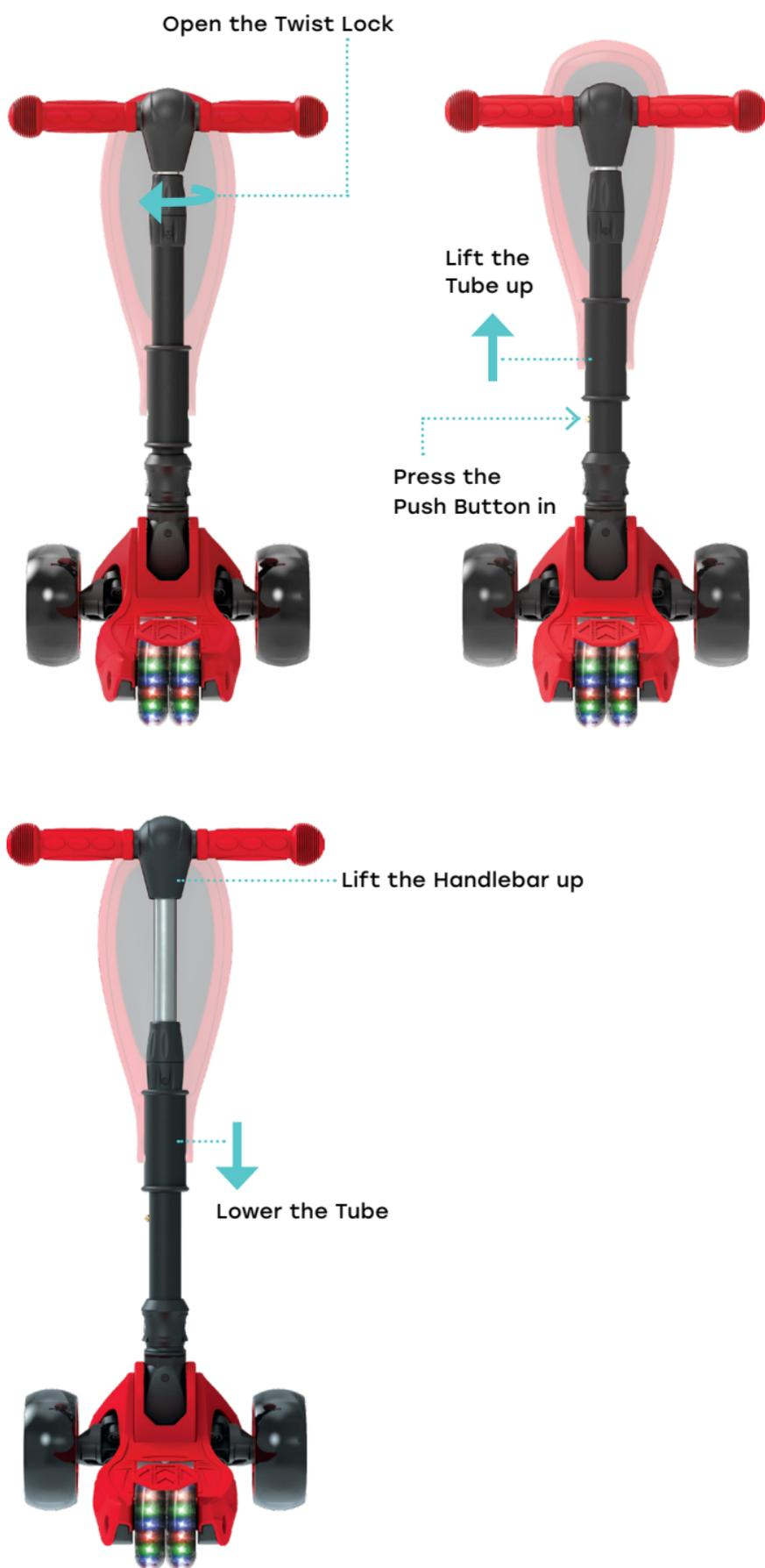
When you hear the Push Button click, close the Twist Lock to lock the Handlebar in place. Make sure the Handlebar is secure.
