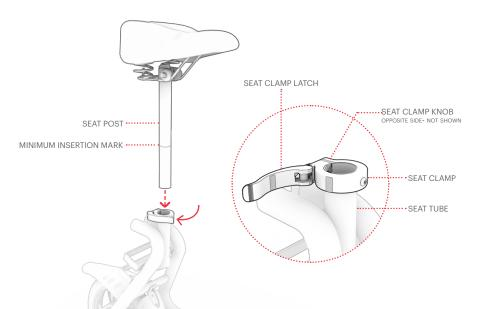
5. RE-TIGHTEN THE KNOB BY TURNING IT CLOCKWISE.
