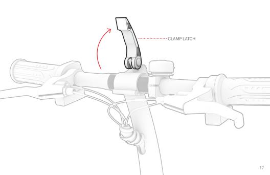
3. ROTATE THE HANDLEBAR FORWARD OR BACKWARDS AS NECESSARY UNTIL THE HANDBRAKES ARE AT THE DESIRED HEIGHT.
