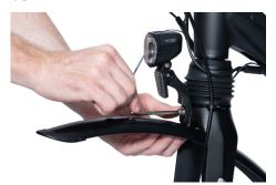
Connect the Fender and Headlight to the Front Fork using the Large Bolt and Washer.
