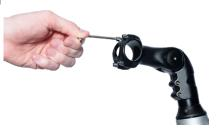
Remove the 4 bolts from the Metal Guard on the Handlebar Stem. Then, remove the Metal Guard. 3.2
