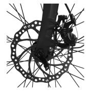
Slide the Quick Release through the Front Tire. Then, place the Spring and Cap back onto the Quick Release.
