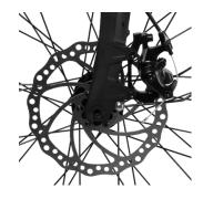
Hook the Fork onto both sides of the tire and slide the Disc Brake into the Disc.
