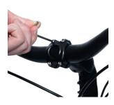
Place the Handlebar into the Handlebar Stem. Make sure the markings on the Handlebar are centered.
