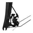
Remove the plastic protector from the Fork. Then, Slide the Front Tire between the Fork. 6.2
