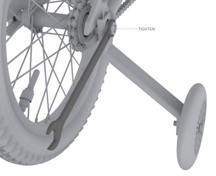
• REPEAT ON THE OTHER SIDE OF THE BICYCLE. ONCE BOTH BRACKETS ARE CONNECTED, TIGHTEN SECURELY
