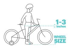
FOR SAFE AND COMFORTABLE RIDING THERE SHOULD BE A CLEARANCE OF AT LEAST 1-3 INCHES BETWEEN THE CROTCH AND THE TOP TUBE OF THE BICYCLE FRAME, WHILE THE RIDER STRADDLES THE BICYCLE WITH BOTH FEET FLAT ON THE GROUND.
