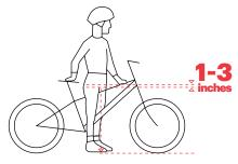
FOR SAFE AND COMFORTABLE RIDING, THERE SHOULD BE A CLEARANCE OF AT LEAST 1-3 INCHES BETWEEN THE CROTCH AND THE TOP TUBE OF THE BICYCLE FRAME WHEN THE RIDER STRADDLES THE BICYCLE WITH BOTH FEET FLAT ON THE GROUND.
