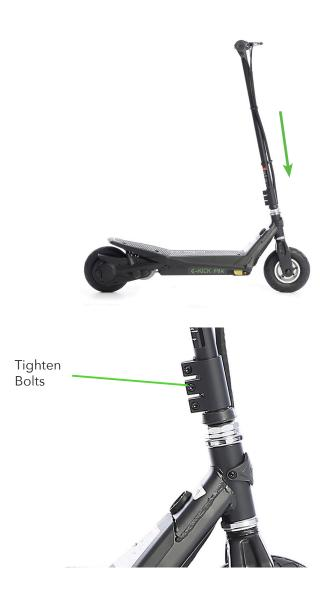
To assemble the Handlebar, first place the Handlebar at the top of the Stem. Align the markings on the Handlebar to those at the top of the Stem so that the Handlebar is centered. Cover the Handlebar with the Cover Plate.
