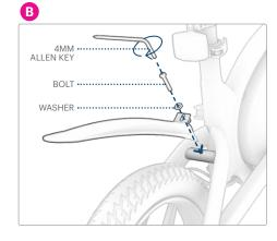
4. TIGHTEN THE BOLT BY TURNING IT CLOCKWISE WITH THE ALLEN KEY. IF APPLICABLE, USE THE WRENCH TO HOLD THE NUT STEADY.
