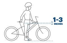
FOR SAFE AND COMFORTABLE RIDING, THERE SHOULD BE A CLEARANCE OF AT LEAST 1-3 INCHES BETWEEN THE CROTCH AND THE TOP TUBE OF THE BICYCLE FRAME WHEN THE RIDER STRADDLES THE BICYCLE WITH BOTH FEET FLAT ON THE GROUND.
