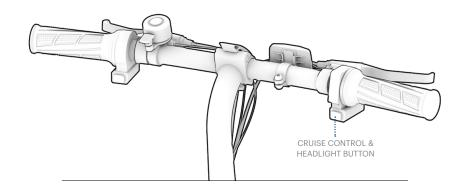
NOTE: USE THE THROTTLE, NOT PEDALING, TO SET THE PACE FOR CRUISE CONTROL.
