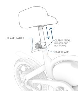
4. CHECK THAT THE SEAT IS SECURE: USE YOUR HAND TO PUT DOWNWARD PRESSURE ON THE SEAT. IF THE SEAT POST SLIPS FURTHER DOWN INTO THE TUBE, BRING IT BACK TO POSITION AND TIGHTEN THE CLAMP FURTHER WITH ADDITIONAL CLOCKWISE TURNS OF THE KNOB. TROUBLESHOOTING: IF YOU CANNOT OPEN AND CLOSE THE LATCH, THE KNOB MAY BE TOO TIGHT. LOOSEN THE KNOB ½ ROTATION AT A TIME UNTIL YOU CAN MAKE USE OF THE LATCH.
