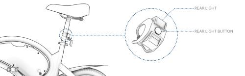
TO CHANGE THE BATTERY: 1. REMOVE THE REAR LIGHT FROM THE SEAT POST BY UNFASTENING ONE ELASTIC STRAP FROM THE HOOK.
