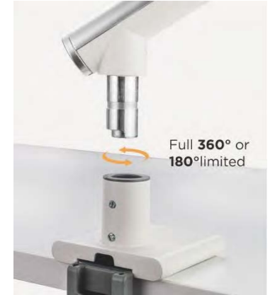
Built-In 180° Rotation Stop for confining the rotation to 180° by tightening the lower screw, which prevents interference with walls or desk partitions
