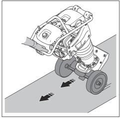
5. Remove the transport device in the opposite sequence.
