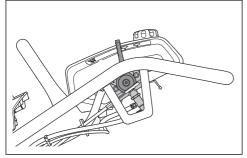
2. If the engine is cold, push the primer bulb 5 times.
