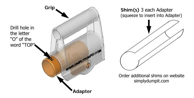
Insert shims one at a time into adapter
