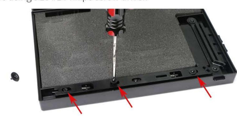
2. Remove the Thumb Lock by carefully unscrewing the two mounting screws and lifting the small end of Thumb Lock up and sliding out of the holes.
