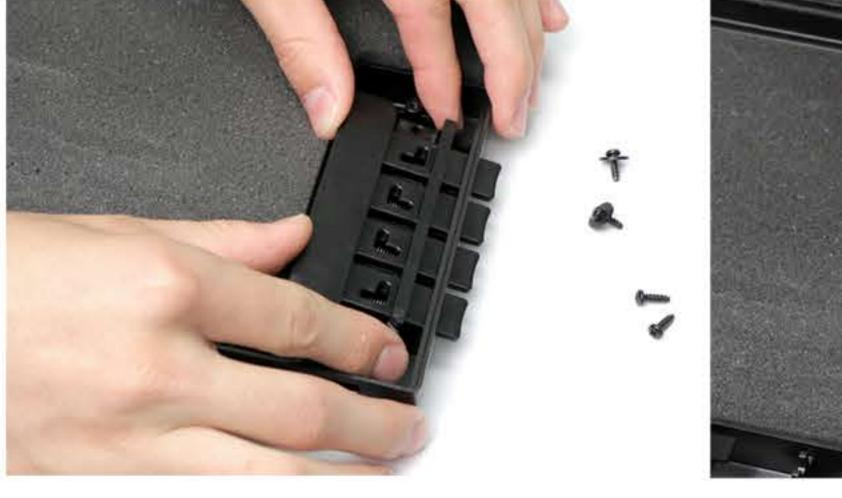
4. There are two types of actuators; "Normally Locked" which must be pressed to unlock the StopBox® and "Normally Unlocked" which are NOT pressed to unlock the StopBox®. Carefully remove actuators intended to be changed by pressing them up away from the chassis.
