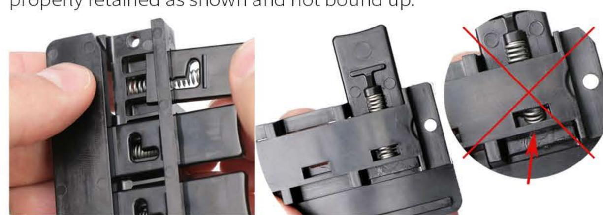
6. While holding the chassis, carefully guide the actuators through the enclosure holes. Press the chassis forward and down to lock into place.
