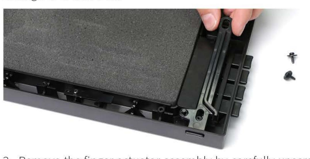
3. Remove the finger actuator assembly by carefully unscrewing the two mounting screws. Using both thumbs press the inside ledge forward and tilt the chassis up as shown. Remove the chassis carefully while the finger actuators are retained in the actuator assembly.
