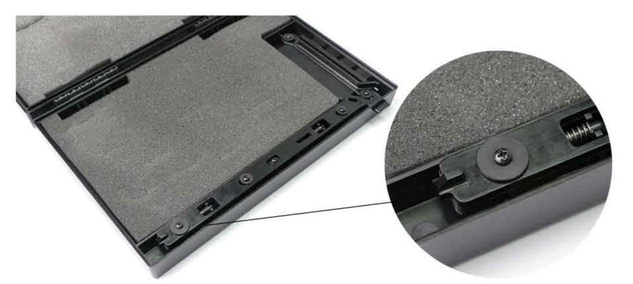
13. Test the functionality of the assembly. Note: the assembly is working correctly when the Lock Bar is held locked back while open and will automatically lock when the enclosure lid is closed.
