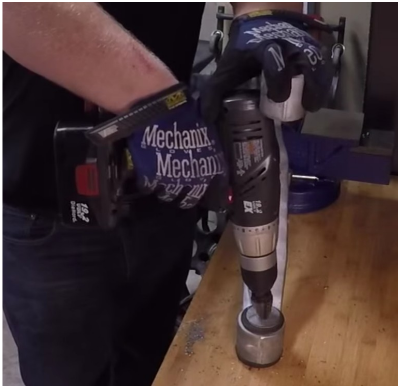
Figure 2. Drilling the bushing washers off.
