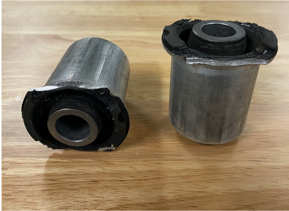
Figure 3. Previously removed bushings showing the cut steel lips.
