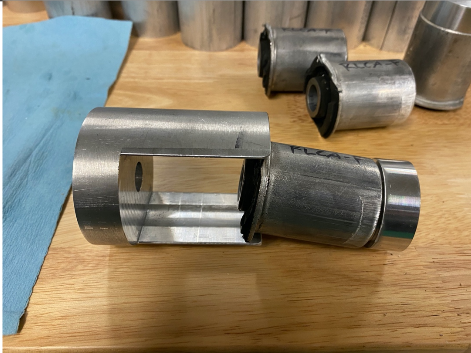
Figure 6. Example of spacer configuration when pressing out a bushing (Note that this image includes preproduction spacers. Your spacers may have a different appearance).
