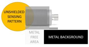
NOTE – WITH UNSHIELDED SENSORS, AN AREA WITHIN THE SENSING PATTERN MUST BE KEPT FREE OF METAL
