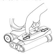
1. Press the tab release button and the brush roll tab pops out.
