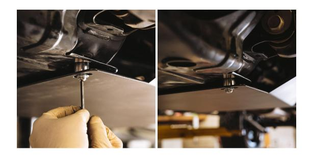
**5.)** Finish it off by tightening down the two rear carriage bolts fully with your 14mm ratcheting wrench, (flex head recommended). Adjust as needed.
