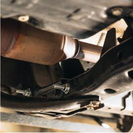
**2.)** Next, remove the two factory rear skid plate bolts with a 12mm socket.
