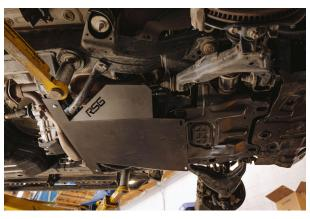
**4.)** Install the included spacers between the factory skid plate and Cat Skid Guard. Use the provided hardware and Allen key to tighten down.
