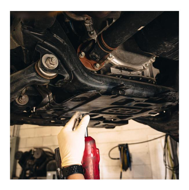
**3.)** Now it is time to lift up the Cat Skid Guard and loosely fit up the two rear carriage bolts to the transmission crossmember.
