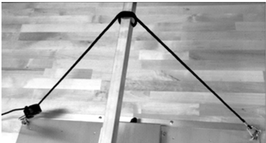
Figure 2 – All mounting points should be connected to the hanging hooks
