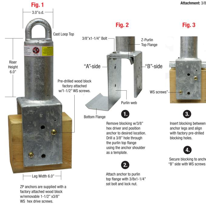
**ZP Anchor Materials:** Riser: Sch 40 3.0" o.d. pipe Loop Top: Q235 Cast steel
