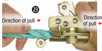
Fig.4.12 Mobility Test Hold connector ring down. Pull lifeline in opposite direction. Lifeline should move freely.
