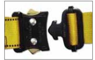
State of the art push release buckles are rated at 5,000 lbs. The unique design requires both tabs to be compressed to release the male end. This feature protects against accidental release.
