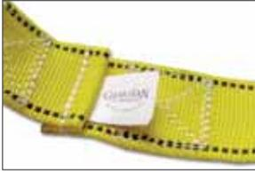
This feature tells the user if the equipment has been loaded in a fall situation. If the indicator is pulled and the full tag is showing, the harness should be removed from service.
