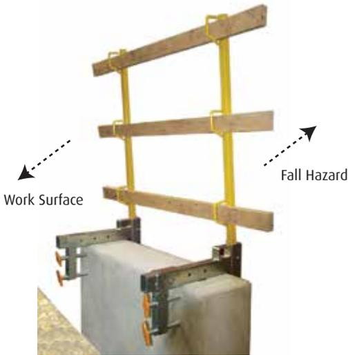
2. Install all guardrails. Guardrails may be 2" x 4" or 2" x 6" construction grade lumber, or compatible snap-on metal rails. If using lumber guardrails, lap guardrails in a continuous direction. Lumber guardrails must overlap a minimum of 12" at each end between consecutive guardrail posts.
