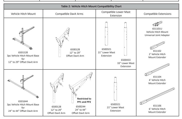
Note: Only one extension or universal joint adapter should be used at a time.
