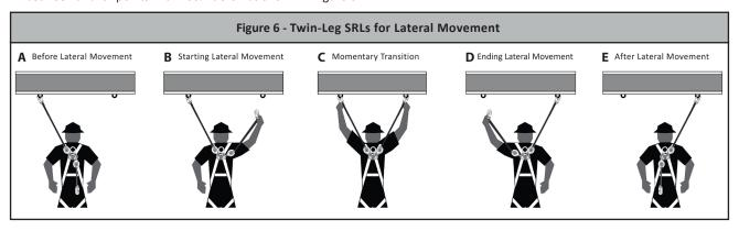
Avoid sudden or quick movements during the normal work operation, as this may cause the SRL pawl system to engage and possibly cause loss of balance, which may cause injury or death. If a fall occurs, the pawl system will engage and lock the lifeline. The EA will deploy to arrest the fall and limit arrest forces on the user.
