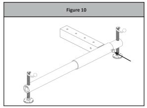
Before inserting the legs into the base center section, refer to the table in Figure 2 to match the Base Position with the Pin Positions of the Davit Arm. To install the Davit Base Legs, ensure the red thumb screws are loosened (turn counter-clockwise). Insert the legs into the base center section and determine the offset your application requires, align the holes and insert the detent pins, Figure 11. Tighten the red thumb screws (clockwise) to ensure are locked in place as shown in Figure 12.
