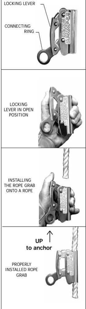
upward through the rope grab while the locking lever is in the up position. When your new location is reached, release the locking lever and the rope grab will lock onto the rope.
