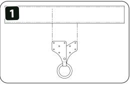
1. Choose location in Wood Truss Member. A qualified person must determine if a specific installation location will meet all ANCHORAGE REQUIREMENTS.
