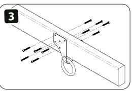
3. Fasten with all ten wood screws (included). Note: To decrease the chance of splitting, Pilot holes (7/64" Ø for soft woods or 1/8" Ø in hard woods) are recommended. If splitting occurs the anchorage connector *must be* moved to a new approved location.
