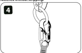
4. Connect personal arrest system (PFAS) to attachment point. PFAS must limit fall arrest forces to 900-lbf (4kN) or less.
