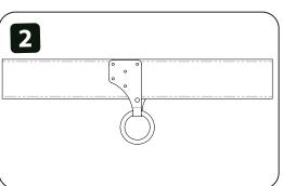
2. Place Anchorage Connector on Wood Truss Member and align. Rivet should be flush with Wood Truss Member. Alignment edge should be perpendicular to length of Wood Truss Member.
