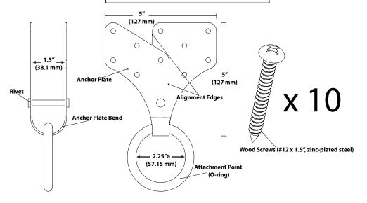
Minimum Breaking Strength (MBS): 1,800-lbf (8kN)
